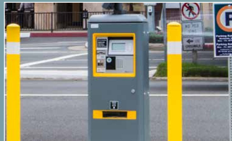
Figure 5.14: Example of a Pay Station (Image Source: Pacific Parking Systems, Inc.)
